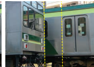
No Rolling Shutter Artifacts with Global Shutter
